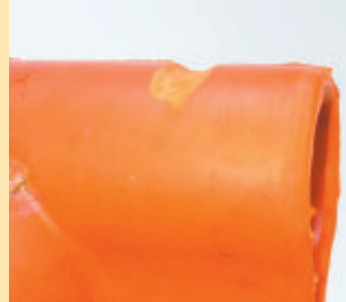
Physical Damage: Rope burns, deep cuts and punctures are cause for rejection.
