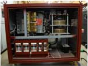
Phenix HC 75 High Current Test set - Preventative maintenance, calibration and certification.
