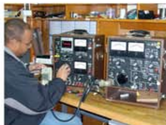
Multi-amp protective relay test set - Repair, calibration and certification.
