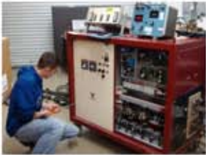
Phenix HC 75 High Current Test set - Preventative maintenance, calibration and certification.
