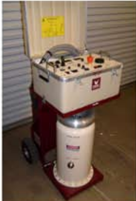
Phenix BK 130 AC Hipot - preventative repair, calibration and certification.
